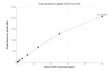
Cytometric bead array standard curve of MP01682-1, TEAD4 Recombinant Matched Antibody Pair, PBS Only. Capture antibody: 84932-1-PBS. Detection antibody: 84932-2-PBS. Standard: Ag3059. Range: 0.781-100 ng/mL
