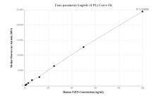
Cytometric bead array standard curve of MP01703-1, USP33 Recombinant Matched Antibody Pair, PBS Only. Capture antibody: 84958-1-PBS. Detection antibody: 84958-3-PBS. Standard: Ag14268. Range: 0.781-100 ng/mL
