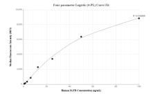
Cytometric bead array standard curve of MP01744-1, EGFR Recombinant Matched Antibody Pair, PBS Only. Capture antibody: 85039-3-PBS. Detection antibody: 85039-2-PBS. Standard: Eg0204. Range: 0.781-100 ng/mL.
