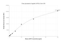
Cytometric bead array standard curve of MP01783-2, ADNP Recombinant Matched Antibody Pair, PBS Only. Capture antibody: 85054-2-PBS. Detection antibody: 85054-1-PBS. Standard: Ag12414. Range: 0.313-40 ng/mL
