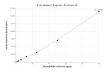
Cytometric bead array standard curve of MP01782-1, ROD1 Recombinant Matched Antibody Pair, PBS Only. Capture antibody: 85061-1-PBS. Detection antibody: 85061-3-PBS. Standard: Ag5172. Range: 1.563-100 ng/mL
