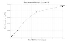
Cytometric bead array standard curve of MP01796-1, STX12 Recombinant Matched Antibody Pair, PBS Only. Capture antibody: 85069-2-PBS. Detection antibody: 85069-3-PBS. Standard: Ag5532. Range: 0.781-100 ng/mL
