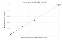
Cytometric bead array standard curve of MP01827-2, Complement factor H/CFH Recombinant Matched Antibody Pair, PBS Only. Capture antibody: 85132-1-PBS. Detection antibody: 85132-3-PBS. Standard: Eg3753. Range: 0.781-100 ng/mL
