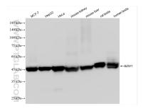
Various lysates were subjected to SDS PAGE followed by western blot with 85655-1-RR (BZW1 antibody) at dilution of 1:10000 incubated at room temperature for 1.5 hours.
