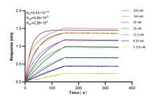
Biolayer interferometry (BLL) kinetic assays of 98130-1-RR against Human L1CAM/CD171 were performed. The affinity constant is 0.243 nM.
