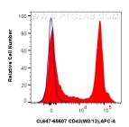
1x10^6 rat splenocytes were surface stained with 0.25ug CoraLite® Plus 647 Anti-Rat CD43 (W3/13) Mouse IgG2a Recombinant Antibody (CL647-65607, Clone: W3/13)(red), or CoraLite® Plus 647 Mouse IgG2a Isotype Control (C1.18.4) (CL647-65208, Clone: C1.18.4) (blue). Cells were not fixed.
