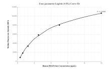
Cytometric bead array standard curve of MP00006-1, PDGFRB Recombinant Matched Antibody Pair, PBS Only. Capture antibody: 82943-2-PBS. Detection antibody: 82943-4-PBS. Standard: Eg0147. Range: 0.313-10 ng/mL
