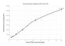
Cytometric bead array standard curve of MP00099-1, TNFR1 Recombinant Matched Antibody Pair, PBS Only. Capture antibody: 83080-1-PBS. Detection antibody: 83080-3-PBS. Standard: Eg0531. Range: 0.625-20 ng/mL
