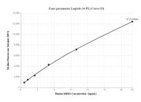
Cytometric bead array standard curve of MP00166-3, MDM1 Recombinant Matched Antibody Pair, PBS Only. Capture antibody: 83141-3-PBS. Detection antibody: 83141-4-PBS. Standard: Ag10541. Range: 0.625-20 ng/mL
