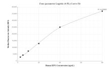
Cytometric bead array standard curve of MP00231-1, RPN1 Recombinant Matched Antibody Pair, PBS Only. Capture antibody: 83250-1-PBS. Detection antibody: 83250-3-PBS. Standard: Ag3576. Range: 2.5-80 ng/mL
