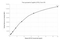
Cytometric bead array standard curve of MP00254-3, MTCO2 Recombinant Matched Antibody Pair, PBS Only. Capture antibody: 83132-4-PBS. Detection antibody: 83132-6-PBS. Standard: SY01099. Range: 0.313-20 ng/mL
