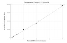
Cytometric bead array standard curve of MP00269-2, EFHD2 Recombinant Matched Antibody Pair, PBS Only. Capture antibody: 83264-2-PBS. Detection antibody: 83264-1-PBS. Standard: Ag35084. Range: 1.25-40 ng/mL
