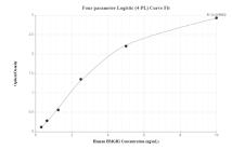
Sandwich ELISA standard curve of MP00311-1, HMGB1 Recombinant Matched Antibody Pair, PBS Only. Capture antibody: 82973-1-PBS. Detection antibody: 82973-3-PBS. Standard: Ag1264. Range: 0.156-10 ng/mL
