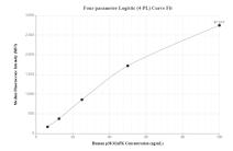
Cytometric bead array standard curve of MP00437-3, p38 MAPK Recombinant Matched Antibody Pair, PBS Only. Capture antibody: 80821-7-PBS. Detection antibody: 80821-4-PBS. Standard: Ag5115. Range: 6.25-100 ng/mL
