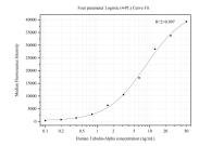
Cytometric bead array standard curve of MP00551-1, Tubulin-Alpha Recombinant Matched Antibody Pair, PBS Only. Capture antibody: 80740-1-PBS. Detection antibody: 80762-1-PBS. Standard:Ag18034. Range: 0.098-50 ng/mL
