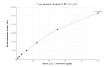
Cytometric bead array standard curve of MP00753-2, ALDX5 Recombinant Matched Antibody Pair, PBS Only. Capture antibody: 83794-3-PBS. Detection antibody: 83794-1-PBS. Standard: Ag19503. Range: 1.56-100 ng/mL
