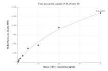
Cytometric bead array standard curve of MP00890-2, CCDC22 Recombinant Matched Antibody Pair, PBS Only. Capture antibody: 83992-3-PBS. Detection antibody: 83992-2-PBS. Standard: Ag9980. Range: 0.313-40 ng/mL
