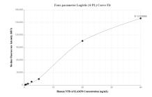
Cytometric bead array standard curve of MP01129-1, NTB-A/SLAMF6 Recombinant Matched Antibody Pair, PBS Only. Capture antibody: 84211-2-PBS. Detection antibody: 84211-1-PBS. Standard: Eg1362. Range: 0.313-40 ng/mL
