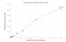
Cytometric bead array standard curve of MP01151-2, KLHDC3 Recombinant Matched Antibody Pair, PBS Only. Capture antibody: 84217-4-PBS. Detection antibody: 84217-2-PBS. Standard: Ag4879. Range: 0.781-100 ng/mL
