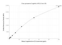
Cytometric bead array standard curve of MP01390-1, Factor IX Recombinant Matched Antibody Pair, PBS Only. Capture antibody: 84533-3-PBS. Detection antibody: 84533-2-PBS. Standard: Eg1045. Range: 0.781-100 ng/mL
