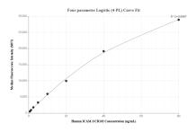
Cytometric bead array standard curve of MP01646-1, ICAM2/CD102 Recombinant Matched Antibody Pair, PBS Only. Capture antibody: 84857-2-PBS. Detection antibody: 84857-1-PBS. Standard: Eg2002. Range: 0.625-80 ng/mL
