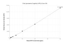
Cytometric bead array standard curve of MP01778-2, BNP Recombinant Matched Antibody Pair, PBS Only. Capture antibody: 85079-3-PBS. Detection antibody: 85079-1-PBS. Standard: Eg1029. Range: 0.625-40 ng/mL
