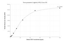
Cytometric bead array standard curve of MP01813-2, STRN Recombinant Matched Antibody Pair, PBS Only. Capture antibody: 85058-3-PBS. Detection antibody: 85058-1-PBS. Standard: Ag15984. Range: 0.781-100 ng/mL
