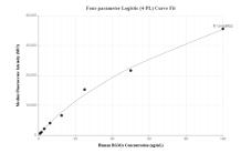
Cytometric bead array standard curve of MP01837-1, RGMA Recombinant Matched Antibody Pair, PBS Only. Capture antibody: 85124-3-PBS. Detection antibody: 85124-2-PBS. Standard: Ag3058. Range: 0.781-100 ng/mL
