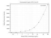
Cytometric bead array standard curve of MP50236-1, PINK1 Monoclonal Matched Antibody Pair, PBS Only. Capture antibody: 68848-1-PBS. Detection antibody: 68848-2-PBS. Standard:Ag19825. Range: 0.781-100 ng/mL.
