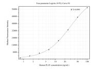
Cytometric bead array standard curve of MP50366-2, PLZF Monoclonal Matched Antibody Pair, PBS Only. Capture antibody: 66672-3-PBS. Detection antibody: 66672-1-PBS. Standard:Ag25180. Range: 0.781-100 ng/mL
