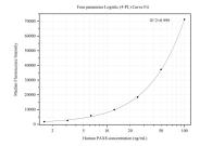
Cytometric bead array standard curve of MP50408-1, PAX8 Monoclonal Matched Antibody Pair, PBS Only. Capture antibody: 68957-1-PBS. Detection antibody: 68957-2-PBS. Standard:Ag20348. Range: 1.563-100 ng/mL
