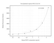
Cytometric bead array standard curve of MP50567-4, PNPT 1 Monoclonal Matched Antibody Pair, PBS Only. Capture antibody: 68309-5-PBS. Detection antibody: 68309-3-PBS. Standard:Ag6290. Range: 0.098-6.25 ng/mL
