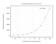
Cytometric bead array standard curve of MP50591-2, SCOT Monoclonal Matched Antibody Pair, PBS Only. Capture antibody: 67836-2-PBS. Detection antibody: 67836-4-PBS. Standard:Ag24792. Range: 0.391-100 ng/mL
