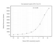
Cytometric bead array standard curve of MP51077-1, CD83 Monoclonal Matched Antibody Pair, PBS Only. Capture antibody: 60744-1-PBS. Detection antibody: 60744-2-PBS. Standard:Ag27435. Range: 0.098-25 ng/mL
